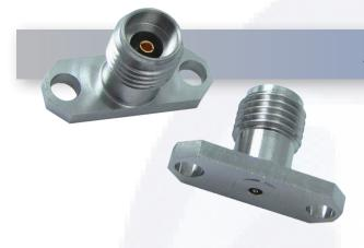
The HASCO **29J-2H-625-012** is a 2.92mm Female Connector with .625" 2-hole flange. It operates from DC to 40 GHz and has a VSWR or 1.15:1 DC to 40Ghz.
