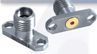
The HASCO **29J-2H-625-12** is a 2.92mm Female Connector with .625" 2-hole flange. It operates from DC to 40 GHz and has a VSWR or 1.25:1 DC to 40Ghz.
