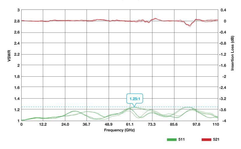
Calibration standard has greater attenuation than the adapter, causing gain. Insertion loss is offset by 2dB.
