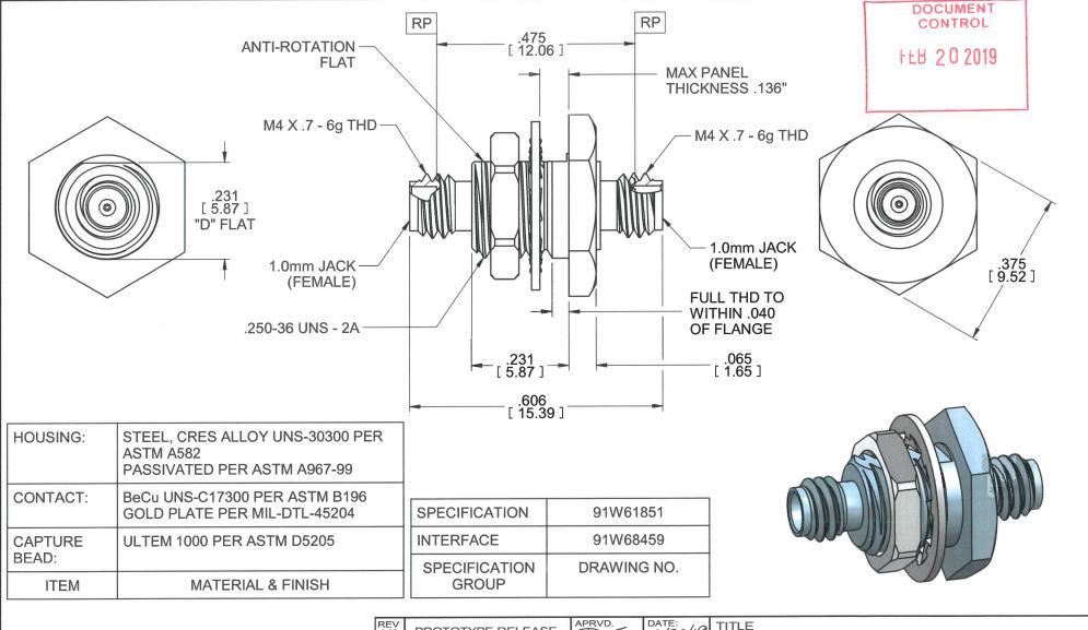
ALL DIMENSIONS ARE IN INCHES. ALL ANGLES ARE IN DEGREES. DIMENSIONS SHOWN IN BRACKETS [XXX] ARE IN MILLIMETERS.
