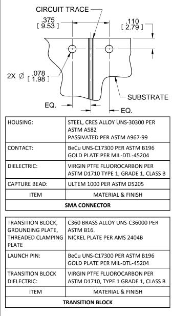
1. ALL DIMENSIONS ARE IN INCHES. ALL ANGLES ARE IN DEGREES. DIMENSIONS SHOWN IN BRACKETS [XXX] ARE IN MILLIMETERS.
