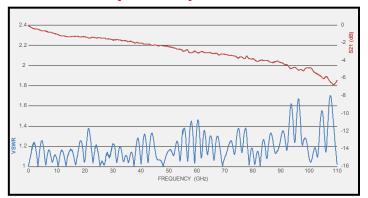
Test data shown are the results from two End Launch connectors and the one inch long test board.
