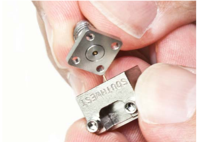
10: Reinstall connector by aligning launch pin into rear of connector.
