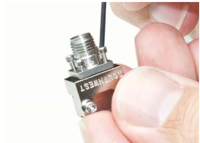
12: Tighten screws following "Mounting Guidelines for Flange Mount Connectors" page 102 in catalog.
