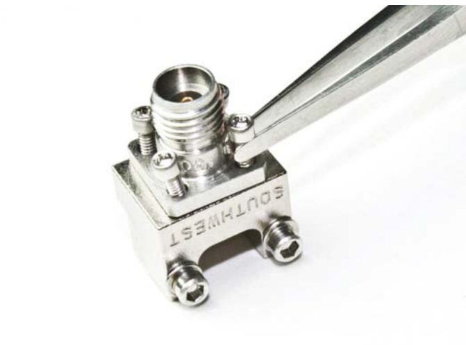
11: Place screws back on connector.
