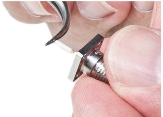
5: Remove pin and dielectric from the connector then proceed to step 7.
