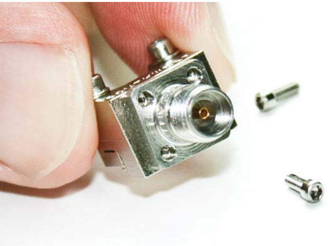
3: Remove all four screws and remove connector.
