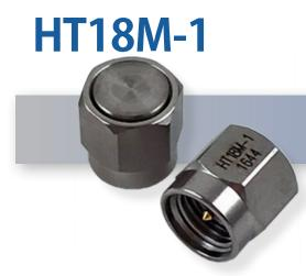
The HASCO **HT18M-1** is an SMA Male RF Load / RF Termination manufactured by HASCO Components. HT18M-1 is rated for operation from DC to 18 GHz and rated for 1 Watt. RF Loads, also known as Terminations are used to prevent signals from flowing back into a transmission line causing unwanted distortion and power loss.
