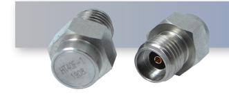
The HASCO **HT40F-1** is an RF termination (also called RF load or dummy load) that operates from DC to 40 GHz and handles up to 1 Watt (CW). Our 2.92mm termination/load has a female gender. HT40M-1 termination offers 1.25:1 max VSWR.
