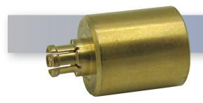
The HASCO **HT6SMPMF-1** is a push on RF Load Termination from HASCO. This RF Load Termination will operate up to 6 GHz and rated for 1 Watt. The SMPM termination was developed for dense connector application, 5G requirements and high speed simiconductor testing.
