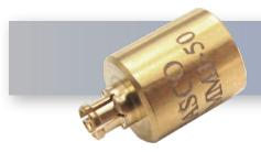
The HASCO **HTMMJ-50** is an RF termination (also called RF load or dummy load) that operates from DC to 50 GHz and handles up to 1 Watt (CW). Our SMPM termination/load has a Female gender. **HTMMJ-50** termination offers 1.4:1 max VSWR DC-50GHz.
