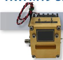
The HWFM19-SF4X15 is a Full Band WR-19 Active Multiplier. This Multiplier can be used as a U-Band Frequency Extender. It operates in frequency from 40 to 60 GHz with an Output Power of +14 dBm min. Multipliers are useful in test labs or in a system. The Output Power is adequate to drive Balance Mixers in Up-Converters and Down-Converters for Transmitters and Receivers.
