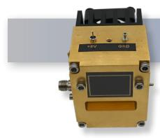
The HWFM22-SF4X15 is a Full Band WR-22 Active Multiplier. This Multiplier can be used as a Q-Band Frequency Extender. It operates in frequency from 33 to 50 GHz with an Output Power of +15 dBm min. Multipliers are useful in test labs or in a system. The Output Power is adequate to drive Balance Mixers in Up-Converters and Down-Converters for Transmitters and Receivers.
