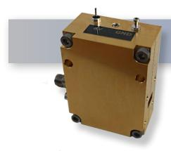
The HWFM28-SF2X23 is a Full Band WR-28 Active Multiplier. This Multiplier can be used as a Ka-Band Frequency Extender. It operates in frequency from 26.5 to 40 GHz with an Output Power of +21 dBm min. Multipliers are useful in test labs or in a system. The Output Power is adequate to drive Balance Mixers in Up-Converters and Down-Converters for Transmitters and Receivers.
