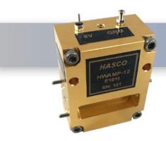
The HWAMP10-W1712 is a Full W-Band Power Amplifier with a gain of +12 dB from 75-105 GHz. This Power Amplifier operates with 7-12VDC. Internal reverse bias protection ensures reliability. This is an excellent full W-Band Power for transmitters, Up-Converters, Radars, and general lab use.
