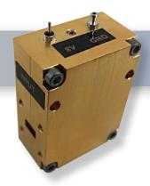
The HWAMP28-KA2222 is a Full Ka-Band Power Amplifier with a gain of +18 dB from 26.5 - 40 GHz. This Power Amplifier operates with 8 VDC. Internal reverse bias protection ensures reliability. This is an excellent full Ka-Band Power for transmitters, Up-Converters, Radars, and general lab use.
