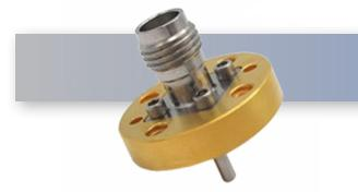
The HASCO HWCA-15VF-EL waveguide to coaxial adapter is manufactured for end-launch (straight) requirements. This adapter is designed for WR-15 waveguide and has a UG385/U compatible flange with a 1.85mm Female connector. A 1.85mm Male version is also available upon request.
