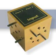
The HASCO **HWMT10-9030T-ER** is a W-band Magic Tee that covers the frequency range of 75 to 105 GHz. A Waveguide Magic Tee is a four-port hybrid coupler and/or power divider with two collinear arms, an E-plane (difference) arm and an H-plane (sum) arm. The Magic Tee offers a 0.3 dB nominal insertion loss and high isolation between the two collinear arms and between the sum and difference arms. All waveguide ports have standard WR-10 waveguides with UG-387/U-M flanges.
