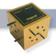
The HASCO **HWMT12-7330T-ER** is a E-band Magic Tee that covers the frequency range of 60 to 86 GHz. A Waveguide Magic Tee is a four-port hybrid coupler and/or power divider with two collinear arms, an E-plane (difference) arm and an H-plane (sum) arm. The Magic Tee offers a 0.3 dB nominal insertion loss and high isolation between the two collinear arms and between the sum and difference arms. All waveguide ports have standard WR-12 waveguides with UG-387/U flanges.
