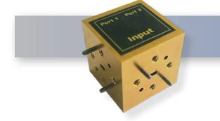
The HASCO **HWMT15-6130T-ER** is a V-band Magic Tee that covers the frequency range of 50 to 72 GHz. A Waveguide Magic Tee is a four-port hybrid coupler and/or power divider with two collinear arms, an E-plane (difference) arm and an H-plane (sum) arm. The Magic Tee offers a 0.3 dB nominal insertion loss and high isolation between the two collinear arms and between the sum and difference arms. All waveguide ports have standard WR-15 waveguides with UG-385/U flanges.
