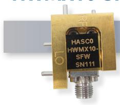
The HWMX10-SFW is a Full W-Band Balanced Mixer. This mixer is designed using the best performance GaAs Schottky beam-lead diodes. These mixers offer excellent low conversion loss and great port to port Isolation. The LO Power required to drive this mixer only needs 10 dBm LO power. The IF operates from DC to 10 GHz. The same mixer can be used as an Up-converter or a Downconverter. This design is very high performance and offered at a great value.
