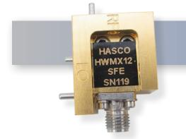
The HWMX12-SFE is a Full E-Band Balanced Mixer. This mixer is designed using the best performance GaAs Schottky beam-lead diodes. These mixers offer excellent low conversion loss and great port to port Isolation. The LO Power required to drive this mixer only needs 13 dBm LO power. The IF operates from DC to 10 GHz. The same mixer can be used as an Up-converter or a Downconverter. This design is very high performance and offered at a great value.
