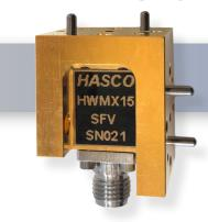
The HWMX15-SFV is a Full V-Band Balanced Mixer. This mixer is designed using the best performance GaAs Schottky beam-lead diodes. These mixers offer excellent low conversion loss and great port to port Isolation. The LO Power required to drive this mixer only needs 13 dBm LO power. The IF operates from DC to 10 GHz. The same mixer can be used as an Up-converter or a Downconverter. This design is very high performance and offered at a great value.
