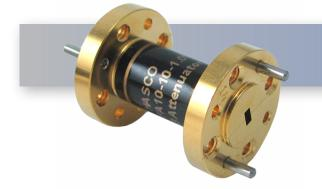
The HASCO WR-10 Millimeter Waveguide Fixed Attenuator **HWFA10-03-1.0** is rated to 0.3 Watts and operates from 75 GHz to 110 GHz. This W-Band, WR-10 attenuator has a fixed attenuation value of 3 dB at center frequency and is constructed with a round UG-387/U-M Flange.
