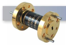
The HASCO WR-10 Millimeter Waveguide Fixed Attenuator **HWFA10-06-1.0** is rated to 0.3 Watts and operates from 75 GHz to 110 GHz. This W-Band, WR-10 attenuator has a fixed attenuation value of 6 dB at center frequency and is constructed with a round UG-387/U-M Flange.
