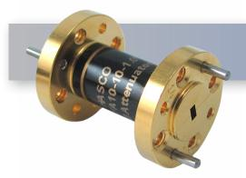
The HASCO WR-10 Millimeter Waveguide Fixed Attenuator **HWFA10-10-1.0** is rated to 0.3 Watts and operates from 75 GHz to 110 GHz. This W-Band, WR-10 attenuator has a fixed attenuation value of 10 dB at center frequency and is constructed with a round UG-387/U-M Flange.
