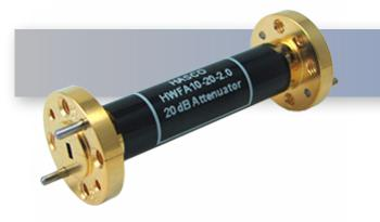
The HASCO WR-10 Millimeter Waveguide Fixed Attenuator **HWFA10-20-2.0** is rated to 0.3 Watts and operates from 75 GHz to 110 GHz. This W-Band, WR-10 attenuator has a fixed attenuation value of 20 dB at center frequency and is constructed with a round UG-387/U-M Flange.
