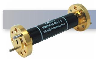
The HASCO WR-10 Millimeter Waveguide Fixed Attenuator **HWFA10-30-2.0** is rated to 0.3 Watts and operates from 75 GHz to 110 GHz. This W-Band, WR-10 attenuator has a fixed attenuation value of 30 dB at center frequency and is constructed with a round UG-387/U-M Flange.
