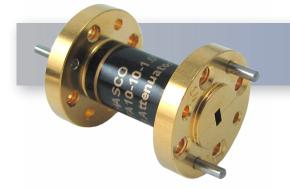
The HASCO WR-12 Millimeter Waveguide Fixed Attenuator **HWFA12-06-1.0** is rated to 0.3 Watts and operates from 60 GHz to 90 GHz. This E-Band, WR-12 attenuator has a fixed attenuation value of 6 dB at center frequency and is constructed with a round UG-387/U Flange.
