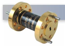
The HASCO WR-15 Millimeter Waveguide Fixed Attenuator **HWFA15-06-1.0** is rated to 0.3 Watts and operates from 50 GHz to 75 GHz. This V-Band, WR-15 attenuator has a fixed attenuation value of 6 dB at center frequency and is constructed with a round UG-385/U-M Flange.
