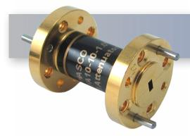
The HASCO WR-15 Millimeter Waveguide Fixed Attenuator **HWFA15-10-1.0** is rated to 0.3 Watts and operates from 50 GHz to 75 GHz. This V-Band, WR-15 attenuator has a fixed attenuation value of 10 dB at center frequency and is constructed with a round UG-385/U Flange.
