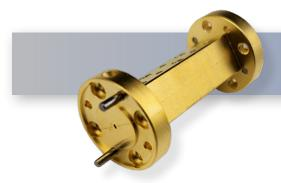
The HASCO WR-3 Millimeter Waveguide Straight Section **HWSS03-2-ER** operates from 220 GHz to 330 GHz. This WR-3, waveguide section is constructed with a Round UG-387/U-M Flange.
