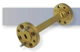
The HASCO WR-5 Millimeter Waveguide Straight Section **HWSS05-2.0-ER** operates from 140 GHz to 220 GHz. This WR-5, waveguide section is constructed with a Round UG-387/U-M Flange.
