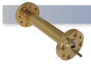
The HASCO WR-10 Millimeter Waveguide Section **HWSS10-2.0-ER** operates from 75 GHz to 110 GHz. This WR-10, W-Band straight section is constructed with a round UG-387/U-M Flange.
