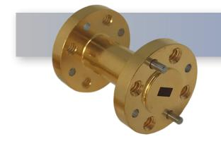
The HASCO WR-12 Millimeter Waveguide Section **HWSS12-1.0-ER** operates from 60 GHz to 90 GHz. This WR-12, E-Band straight section is constructed with a round UG-387/U Flange.
