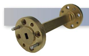
The HASCO WR-12 Millimeter Waveguide Straight Section **HWSS12-2.0-ER-1** operates from 60 GHz to 90 GHz. This WR-12, E-Band waveguide section is constructed with a Round UG-387/U-M Flange.
