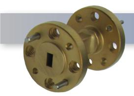
The HASCO WR-15 Millimeter Waveguide Straight Section **HWSS15-1.0-ER-1** operates from 50 GHz to 75 GHz. This WR-15, V-Band waveguide section is constructed with a Round UG-387/U-M Flange.
