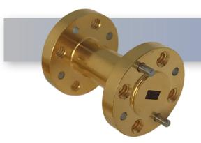
The HASCO WR-15 Millimeter Waveguide Section **HWSS15-1.0-ER** operates from 50 GHz to 75 GHz. This WR-15, V-Band straight section is constructed with a round UG-385/U Flange.
