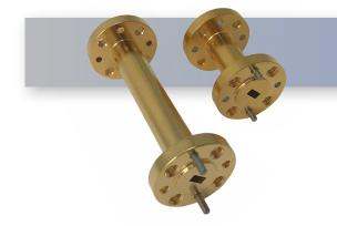
The HASCO WR-19 Millimeter Waveguide Straight Section **HWSS19-2.0-ER** operates from 40 GHz to 60 GHz. This WR-19, U-Band waveguide section is constructed with a Round UG-383/U-M Flange.
