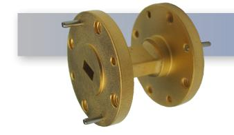
The HASCO WR-22 Millimeter Waveguide Straight Section **HWSS22-1.0-ER** operates from 33 GHz to 50 GHz. This WR-22, Q-Band waveguide section is constructed with a Round UG-383/U-M Flange.
