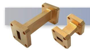
The HASCO WR-28 Millimeter Waveguide Straight Section **HWSS28-2.-ES** operates from 26.5 GHz to 40 GHz. This WR-28, Ka-Band waveguide straight section is constructed with a Square UG-599/U Flange.
