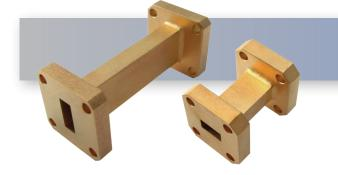
The HASCO WR-34 Millimeter Waveguide Straight Section **HWSS34-1.5-ES** operates from 22 GHz to 33 GHz. This WR-34, waveguide straight section is constructed with a Square UG-595/U-M Flange.
