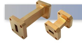
The HASCO WR-34 Millimeter Waveguide Straight Section **HWSS34-2.0-ES** operates from 22 GHz to 33 GHz. This WR-34, waveguide straight section is constructed with a Square UG-595/U-M Flange.
