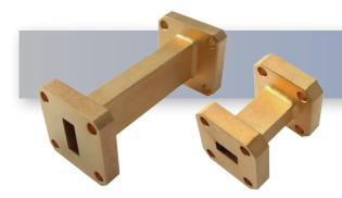
The HASCO WR-42 Millimeter Waveguide Straight Section **HWSS42-1.0-ES** operates from 18 GHz to 26.5 GHz. This WR-42, K-Band waveguide straight section is constructed with a Square UG-595/U Flange.
