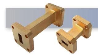
The HASCO WR-42 Millimeter Waveguide Straight Section **HWSS42-1.5-ES** operates from 18 GHz to 26.5 GHz. This WR-42, K-Band waveguide straight section is constructed with a Square UG-595/U Flange.
