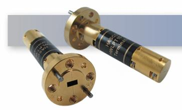
The HASCO WR-10 Millimeter Waveguide, W-Band Termination **HWLPT10-ER** is rated to 0.3 Watts and operates from 75 GHz to 110 GHz. This WR-10, W-Band termination is constructed with a circular UG-387/U-M Flange.
