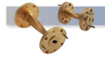
The HASCO WR-6 Millimeter Waveguide 90° Twist **HWTW06-2.5-ER** operates from 110 GHz to 175 GHz. This WR-6, D-Band waveguide 90° Twist is constructed with a Round UG-387/U-M Flange.
