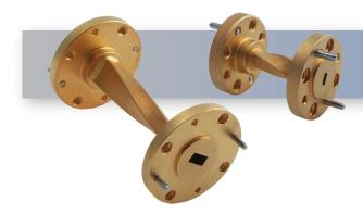
The HASCO WR-8 Millimeter Waveguide 90° Twist **HWTW08-1-ER** operates from 90 GHz to 140 GHz. This WR-8, F-Band waveguide 90° Twist is constructed with a Round UG-387/U-M Flange.
