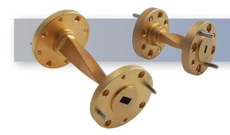
The HASCO WR-10 Millimeter Waveguide 90° Twist **HWTW10-2.5-ER** operates from 75 GHz to 110 GHz. This WR-10, W-Band waveguide 90° Twist is constructed with a Round UG-387/U-M Flange.
