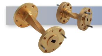
The HASCO WR-15 Millimeter Waveguide 90° Twist **HWTW15-1-ER** operates from 50 GHz to 75 GHz. This WR-15, V-Band waveguide 90° Twist is constructed with a Round UG-385/U Flange.
