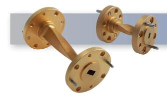
The HASCO WR-19 Millimeter Waveguide 90° Twist **HWTW19-1-ER** operates from 40 GHz to 60 GHz. This WR-19, U-Band waveguide 90° Twist is constructed with a Round UG-383/U-M Flange.
